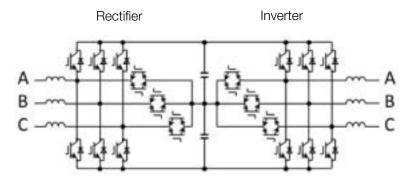
Use of RB-IGBT's reduces parts count and switching losses
