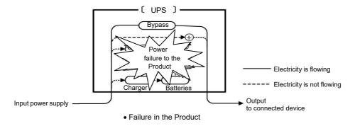
Electricity flow during automatic bypass operation
