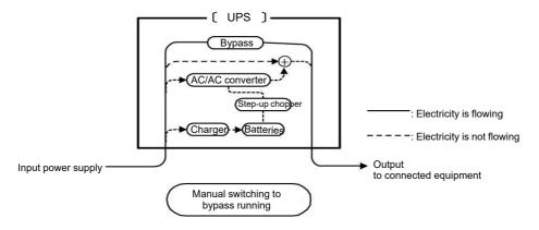
Electricity flow during manual bypass operation
