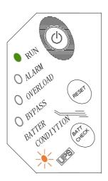
**5.** The battery check takes 5 seconds. After that, if the battery is normal, the BATTERY CONDITION LED (green) on the front of the UPS will again indicate the battery charge level, and the UPS will return to the normal operation.
