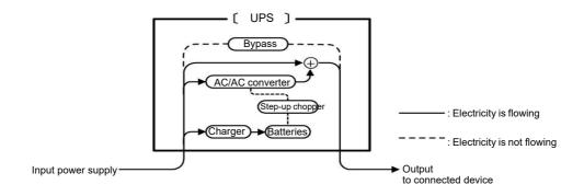
Electricity flow during normal operation
