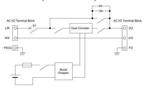
Refer to "Preparation before connection item 2 in 3.2 Connection of cables" (N/S and n/V are neutral terminals.)
