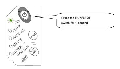
3. AC voltage is output from the AC outlet or the output terminal block. The RUN LED (green) on the front of the UPS lights up. The BATTERY CONDITION LED (green) on the front of the UPS indicates the battery charge level by the lighting type.
