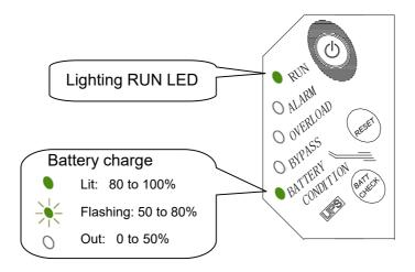
4. The battery check is performed automatically.
