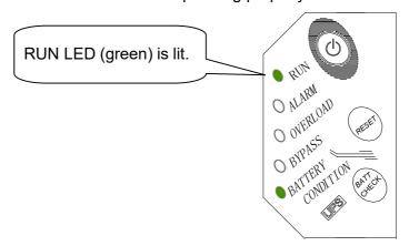
When all the LEDs on the front of the UPS are off, turn on the UPS and proceed to step 2. For details, refer to Chapter 4.1 "Turning on the UPS". Also refer to Chapter 6 "Troubleshooting".
