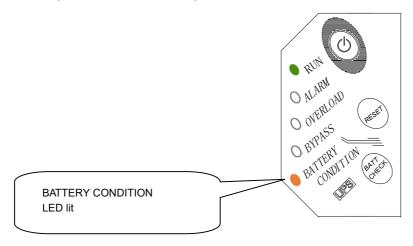
• When the backup time of the battery has been lowered to 3 minutes or less (at the rated load)
