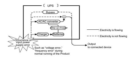
Electricity flow during battery operation
