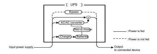
Electricity flow during normal operation
