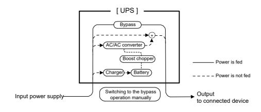
Electricity flow during automatic bypass operation
