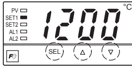
Alarm 1 setpoint (SET1) display
